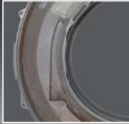
Dirt behind the front cover of the outer tub
